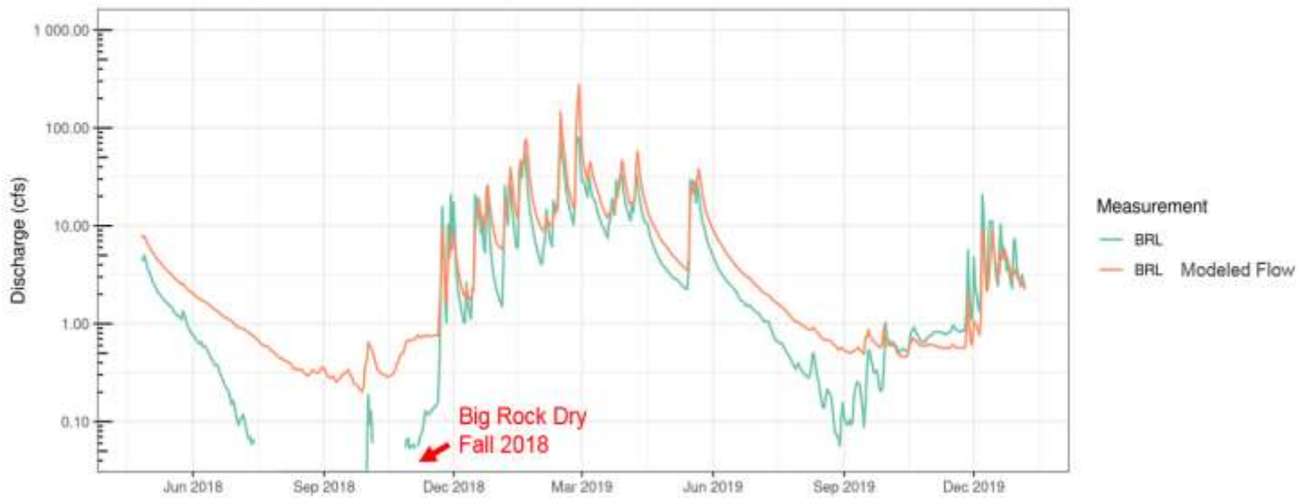
Figure 42. Chart of actual flow of Big Rock Creek versus simulated flow generated by the VELMA model for June 2018 through December 2019.
