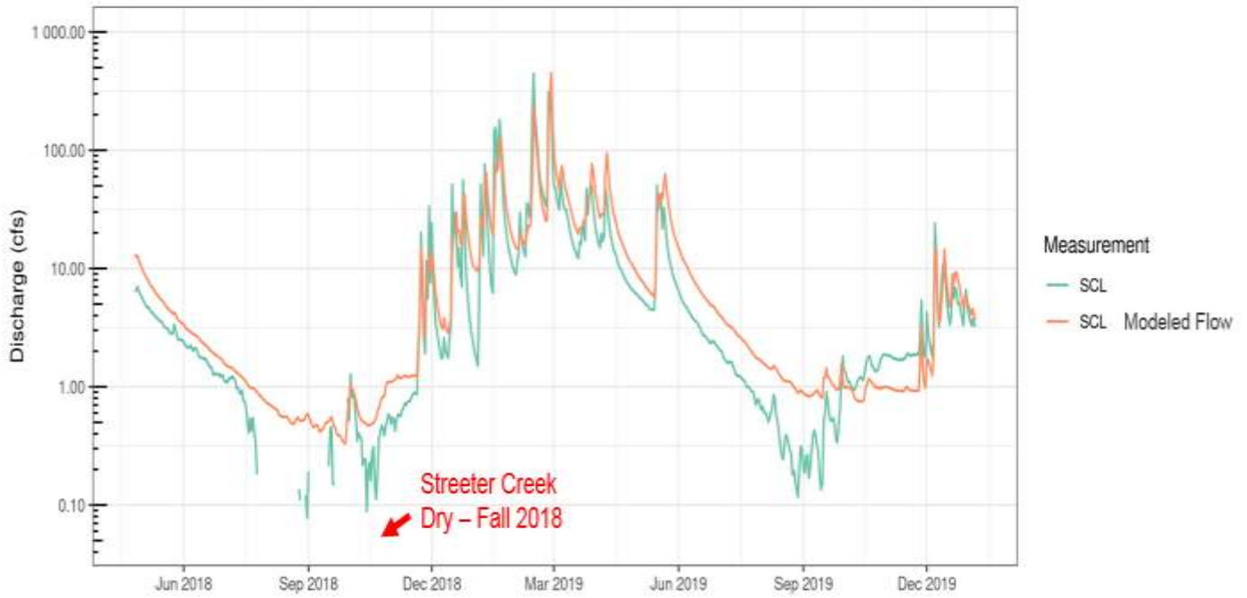
Figure 41. Chart of actual flow of Streeter Creek versus simulated flow generated by the VELMA model for June 2018 through December 2019.
