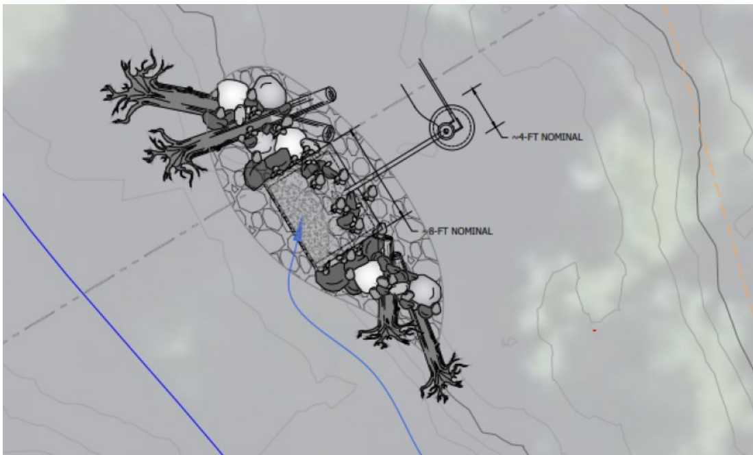
Figure 16. Intake system at Streeter Creek POD that will include fish habitat enhancement structures. By Stillwater Sciences (2022).
