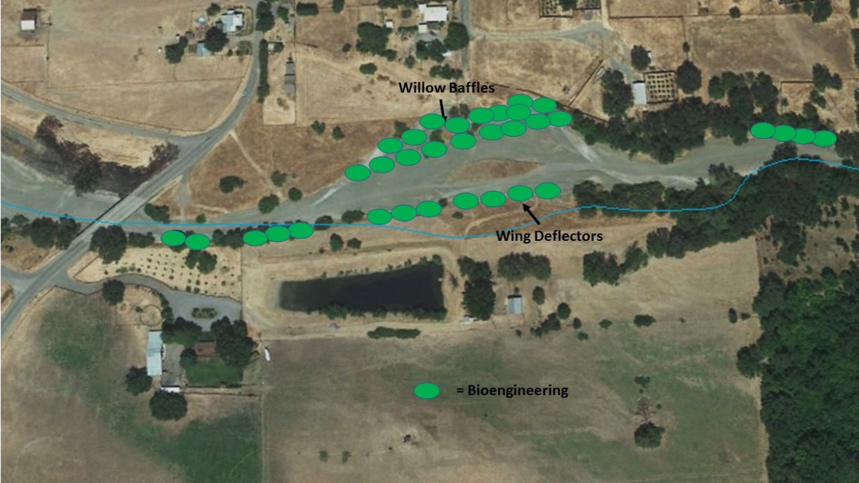
Figure 11. Recommended treatment for Town Creek channel downstream of Airport Road bridge.
