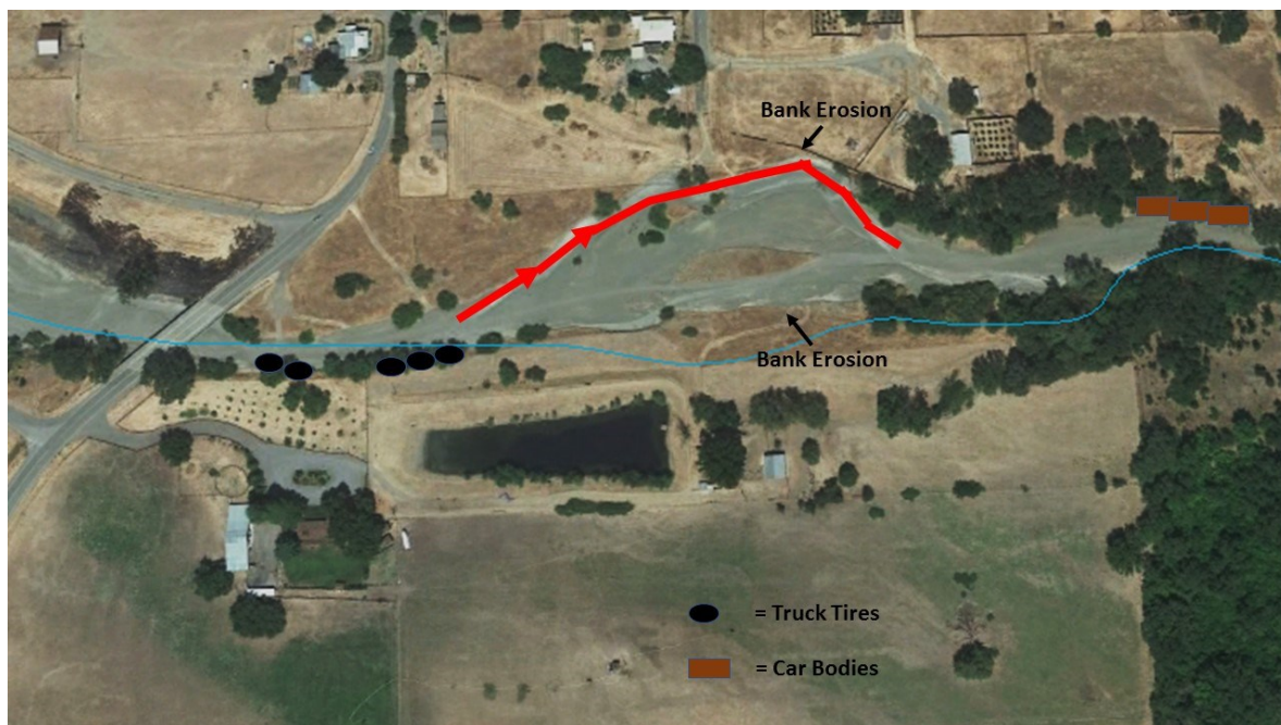
Figure 7. Town Creek reach below Airport Road with current channel (red line), areas of eroding banks, and locations of car bodies and truck tire bank stabilization.
