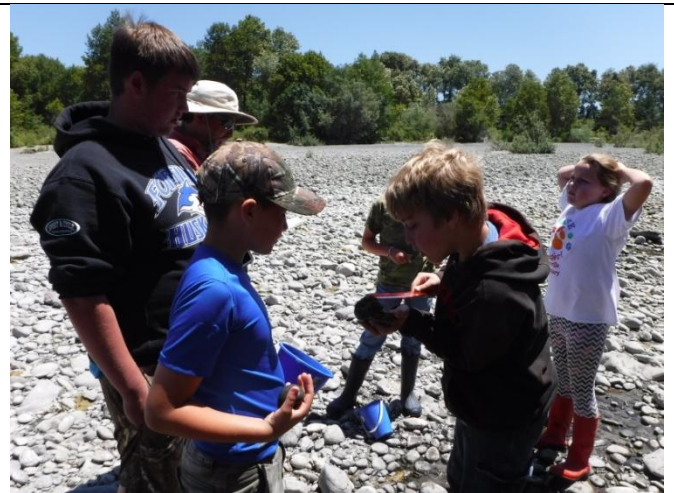
Students measure rock size to determine D-50.
