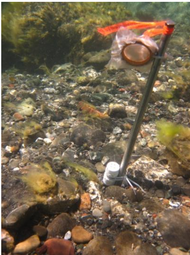
Figure 9 Alderpoint SPATT at top and encased I-Button temperature gauge below.
