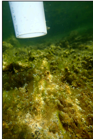
Figure 8. PVC pipe delimiter about to be placed on a patch of benthic algae. Only algae inside the delimiter were collected.
