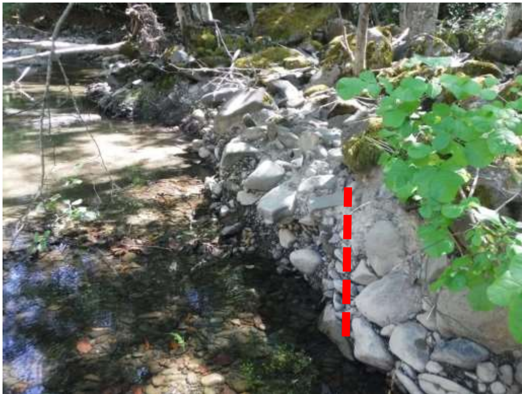
Figure 12. Cross section of cobble terrace in place since 1964 and more than 2 feet of incision in 2016 WY.
